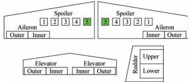
Fig. 1 Schematic of primary flight control surfaces.
