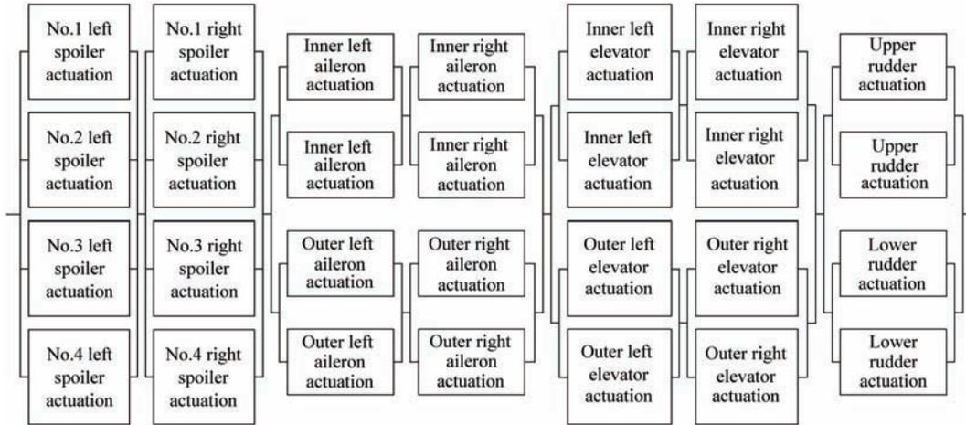
Fig. 2 Safe reliability block diagram of the whole FCAS.
